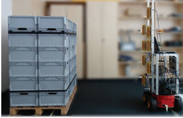
Figure 11. A mobile robot platform equipped with a UHF-RFID MIMO system and a computer generates an aperture, that is, a straight line of 3.2 m, along plastic boxes labeled with tags. The real tag positions are known and are compared to the estimated positions after the signal processing.
