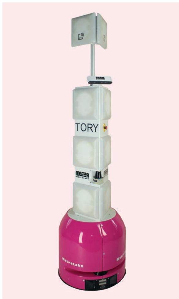
Figure 1. A mobile robot platform is equipped with a UHF-RFID reader that has multiple antennas for automatic and autonomous stocktaking in warehouse applications.
